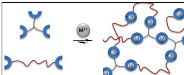
Schematic of supramolecular metallopolymer blends comprised of linear and branched building blocks.
